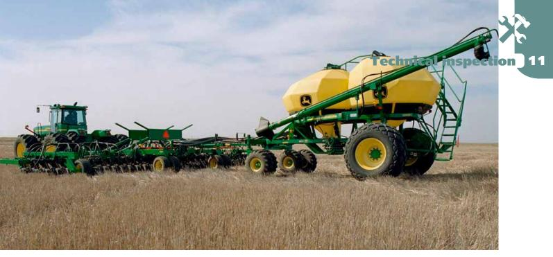
seeding in no-till conditions. This tool is equipped with two rows of openers. The unique one-disc opener allows achieving ideal depth control and seed packing on any soil type. The active hydraulic system adds up to 181 kg of pressure to each opener. It ensures the consistent depth of seed packing. This machine can implement seed and fertiliser in one pass. All drills manufactured at the John Deere factory in Orenburg can be subsidised as machinery assembled in Russia.
