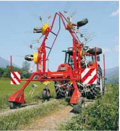
operating condition is 7.85 m. The HIT 800 AZ agitator has a particularly short bracket. The centre of gravity is located very close to the tractor, which reduces strain on the front bridge. The small rotor diameter (130 cm) ensures excellent adaptation to the surface features, better fodder making and regular distribution.
