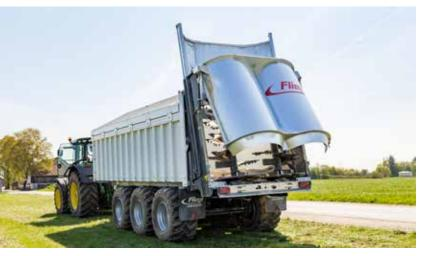
high-capacity spreader with a milling tool made of 400 HB steel, a protective grille to prevent ingress of foreign bodies and a high-performance gearbox and cylinder.
