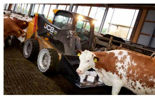
1' buckets. In response to the increasing responsibilities of loaders on livestock farms, the range of implements has been expanded to include manure forks and silage cutters.
