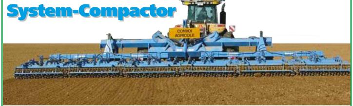
System-Compactor is an ideal tool for preparing a well loosened, smoothly tilled and double-compacted seed bed for cereal crops, sugar beetroots and rape.
