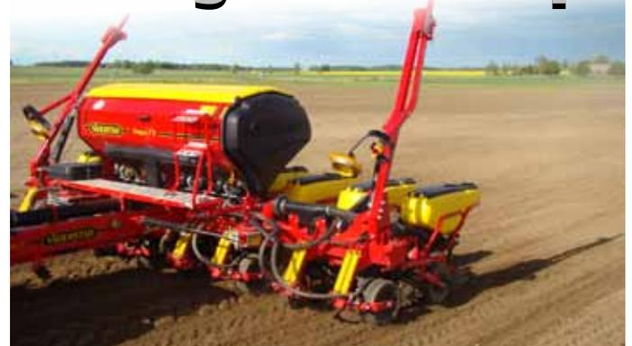
The Tempo F8 Vaderstad seeder unique batcher operating under the high pressure. This minimises the vibration impact and farming technologies, Agrosalon maintains exceptionally high seed introduction precision despite high speed and irregularities of soil.
