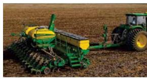
grain bins or a central distribution system. The seed-out sections MaxEmerge Pro – Series XP, jointly with the central distribution system, ensure seeding precision. The movable chassis design ideally follows the terrain profile. According to Yevgeny Manzhurin, head of the department of equipment orders, EkoNiva-Tekhnika, this is a multi-role machine. It is ideally suited for use by farms in the Central, Region, Black Earth Zone and Siberian territories.
