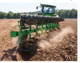
material allowing the plough to operate in adverse field conditions. The model 3910 can have 9 to 13 casings. It performs well in couple with JD 8R and 9R tractors, engine capacity 310 to 460 hp. The plough 3910 has two front bearing wheels and one rear support wheel. They guide the plough over the furrow, which makes it possible to maintain the set tilling depth. Due to its strong design, the plough can operate in all weather conditions.
